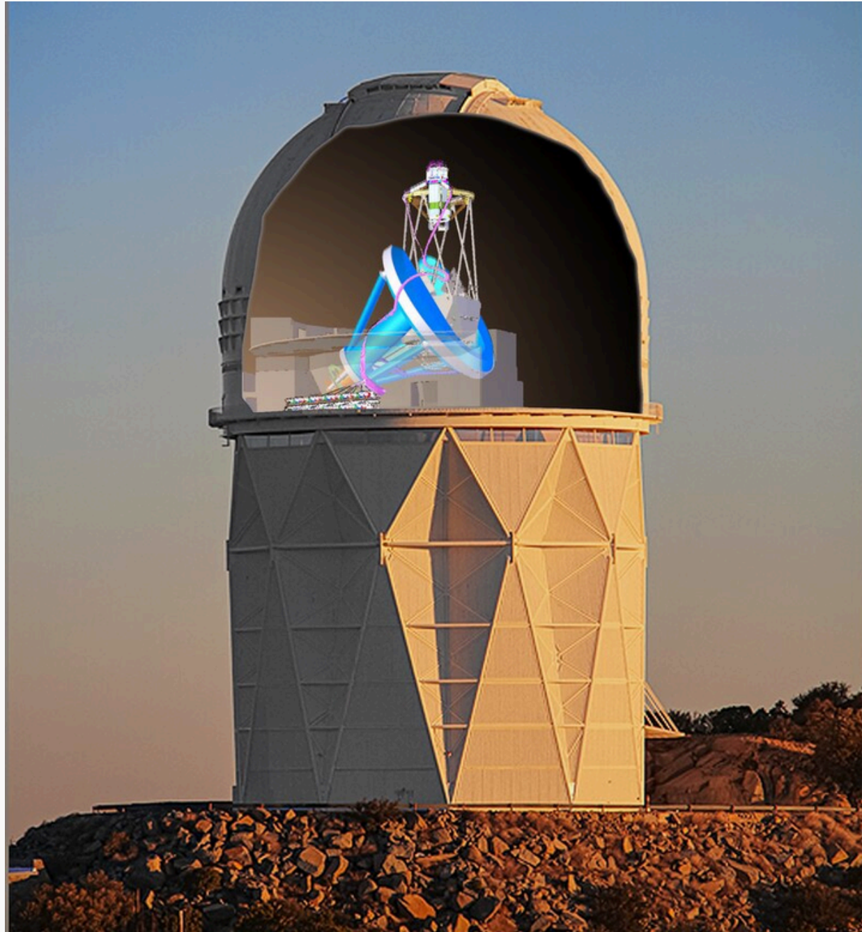
DESI installed on the Nicholas U. Mayall 4-meter Telescope at Kitt Peak National Observatory
