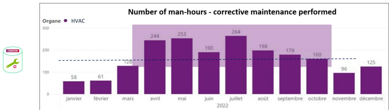
Fig. 7. Correlation between man-hours in corrective maintenance and extended season.
